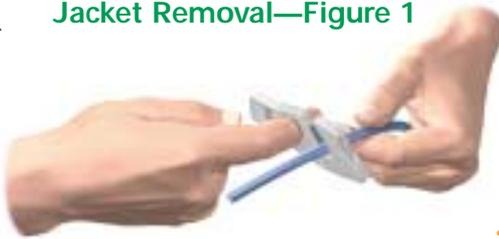
DataTwist: Insert cable into the cutting area and rotate tool at least one complete turn. Remove the jacket end.
