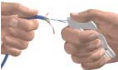
Holding the cable in one hand, with the hand holding the tool, pull the tool away from you, allowing the pick to separate the conductors of the pair.
