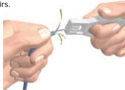
Insert each twisted pair into the appropriate slot. Rotate the tool and/or the pair in the direction opposite of the twist to prevent stripping the conductor insulation. Continue insertion to match the desired length of untwisted section.
