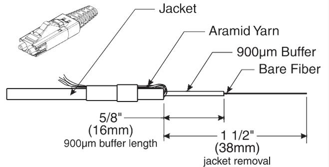
The plug side is not intended to be terminated using 900µm buffered fiber.
